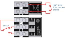
Relay Output Specification: 16Amax resistive load 10Amax inductive load (at 250Vac)
