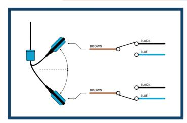
NOTE: To successfully install a float switch, ensure that the float switch is tethered or weighted unless it is internally weighted.
