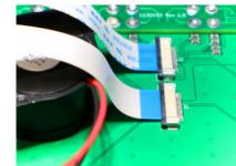
Fit the cables and ensure the blue marks are parallel to the connector J1 & J2
