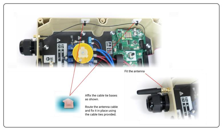
**NOTE:** The antenna cable placement is designed to stay clear of potential high voltages from incoming mains and external circuitry on relay outputs.
