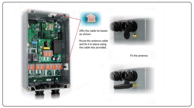
**NOTE:** The antenna cable placement is designed to stay clear of potential high voltages from incoming mains and external circuitry on relay outputs.
