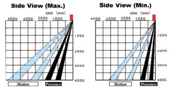
• Outer 3 rows can be deleted one by one using dipswitches.
