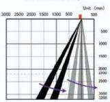
Outer 4 rows can be deleted one by one using dip switches. Outer 2 rows and inner 3 rows can be angled separately using mechanical lever.
