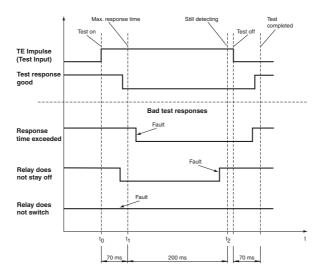
The door controller sends signals to the sensor at the times  $t_1 \mbox{ and } t_2.$
