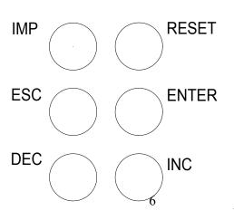
All control parameters and program functions are access via the 6 button keypad. Access is in 3 distinct levels
