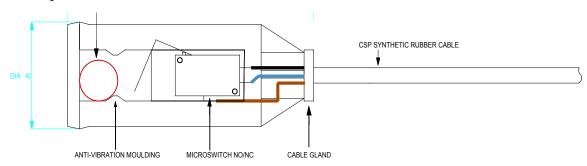
The micro-switch assembly inside the float, axially mounted in line with the weight, changes contacts according to the float's position, as in the diagram below. Therefore as the liquid level drops or rises slowly, a pump or flow control suitably connected, can be switched in or out to maintain an average level of the liquid. By connecting only one side of the switch, the unit can be also used to fill or empty the tank as required.
