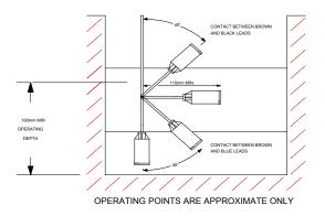
Connection diagram for automatically emptying tank
