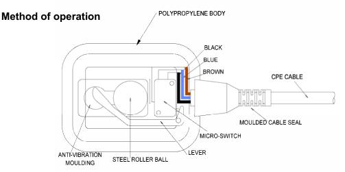
The micro-switch assembly inside the float, axially mounted in line with the weight, changes contacts according to the float's position, as the diagram below.
