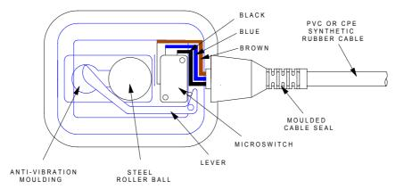
The micro-switch assembly inside the float, axially mounted in line with the weight, changes contacts according to the float's position, as in the diagram below. Therefore as the liquid level drops or rises slowly, a pump or flow control suitably connected, can be switched in or out to maintain an average level of the liquid. By connecting only one side of the switch, the unit can be also used to fill or empty the tank as required.
